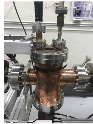
Figure 6: Cavity installed in beamline
