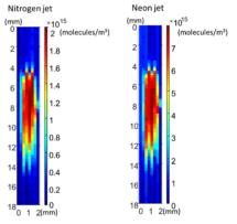
Figure 3: Jet density measurement with the system described in Fig. 2. The inlet pressure for both gases is 5 bar. The density is measured 242 mm away from the interaction point with the 3<sup>rd</sup> skimmer at a 90° angle.
