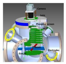
Figure 4: Interaction chamber for gas-jet based IPM beam profile monitor at CI.
