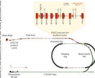
Figure 2: Schematic of the ATF2 with the FONT extractionline feedback system highlighted, showing BPMs P1, P2 and P3 and kickers K1 and K2 [8].
