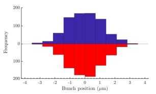
Figure 5: Measured (blue) and predicted (red) bunch positions at P1, with standard deviations of  $1.16 \, \mu m$  and  $1.10 \, \mu m$  respectively.
