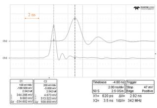
Figure 4: Oscilloscope waveforms from a testbench setup without (Ch1) and with (Ch2) the prototype processor.
