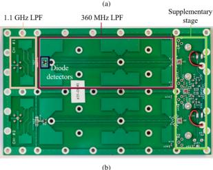
Figure 3: (a) Schematic and (b) photograph of the processor with the diode detectors and LPFs highlighted. (b) also shows the supplementary stage required to interface the processor with the ATF2 FONT system.
