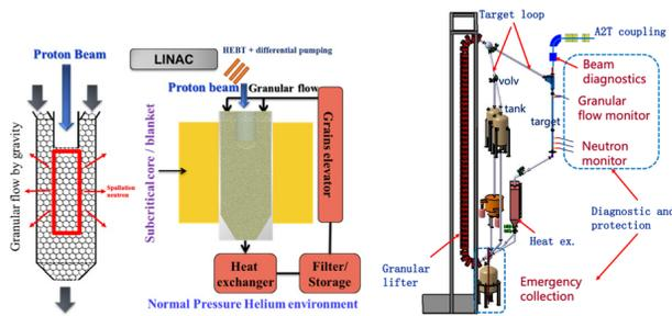
Figure 4: The principle and setup of granular target.
