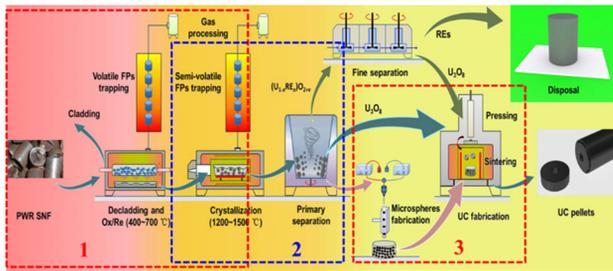
Figure 10: Technical route of reprocessing and fabrication for the spent nuclear fuel.
