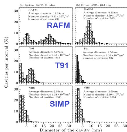
Figure 9: Comparison of cavity formation in different steels under same ion beam irradiation.
