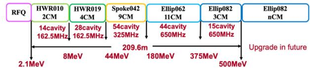
Figure 3: Structure of superconducting liac.
