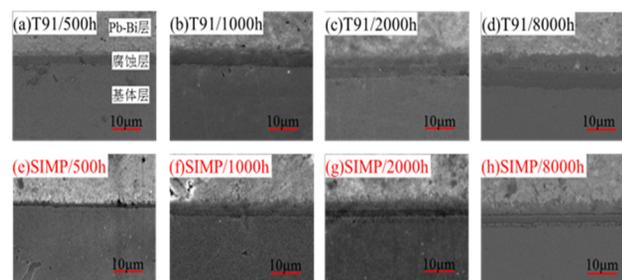
Figure 8: SEM micrograph of cross-sections of SIMP and T91 steels after exposing to LBE with saturated oxygen at 450°C for different time.
