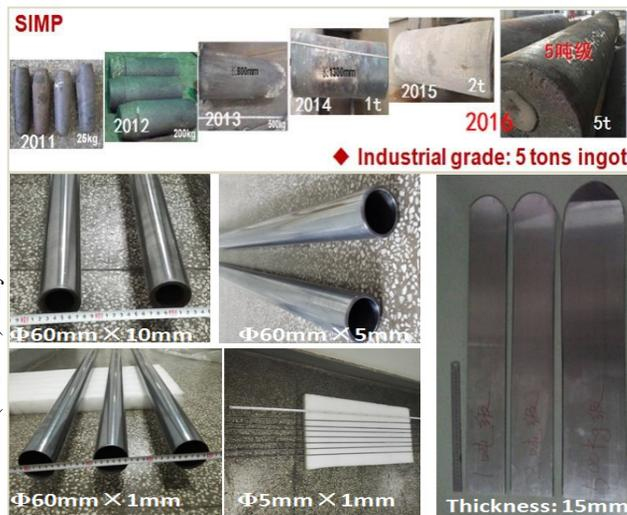
Figure 7: Progress of smelting, casting and mechanical processing of SIMP steel.
