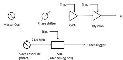
Figure 5: Synchronization diagram of RF and fs Laser system.
