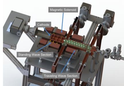
Figure 2: Hybrid gun layout, horizontal cut, marked are the standing wave and traveling wave sections, as well as the cathode location and the magnetic solenoid
