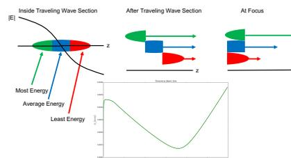
Figure 3: Conversion of applied velocity bunching by the traveling wave section of the gun, to a density bunching after a drift. Green line shows longitudinal compression of the e-bunch.
