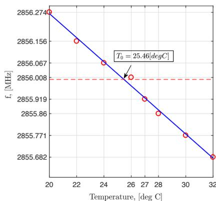
Figure 4: Gun mode frequency (S21) vs temperature of RF structure. Dashed red line marks the required operational frequency (2856 MHz)
