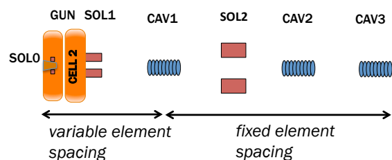
Figure 3: Photoinjector layout used for studies of beam dynamics up to an energy of \sim 20 MeV.
