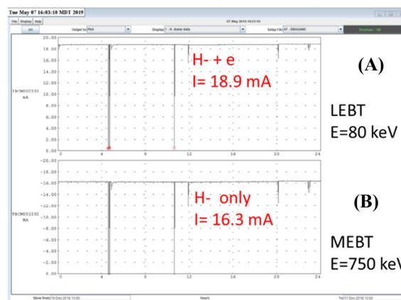
Figure 2: 24 hours charts of stable beam currents recorded at  $H^-$  beam injector: LEBT (A) and MEBT (B).
