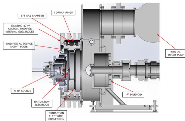
Figure 4: Cross section of SNS RF ion source with 80 kV extraction electrostatic column and two solenoid LEBT is shown.
