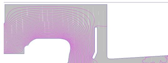
Figure 5: The geometry of the selected electron gun.
