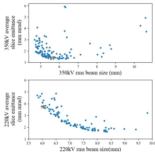
Figure 4: Plots of the objective values of the final solutions showing the average slice emittance against rms beam size for both of the operational voltages. The selected solution is marked as in orange. The x axis of the 220 kV plot is zoomed in for clarity but two solutions with large rms beam size are no longer visible.
