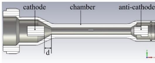
Figure 3: Cold cathode ion source model for simulation.
