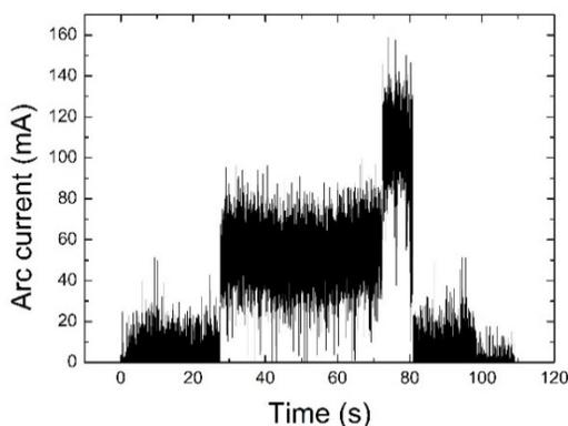
Figure 8: Arc current waveform under 1400V arc voltage.
