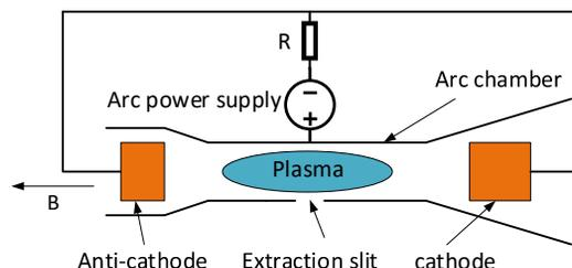
Figure 1: Structure diagram of cold cathode ion source.
