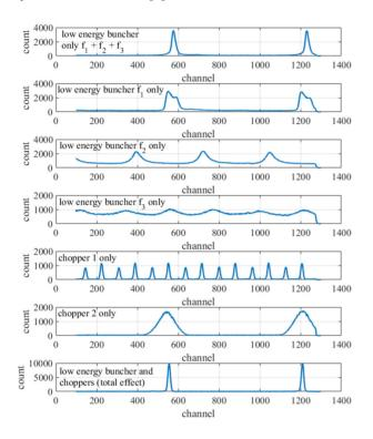
Figure 7: Effect of each component of the pulsing system on the beam timing profile for a 120 keV injection and 75 MeV 160+6 beam (0.1634 ns per channel).
