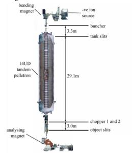
Figure 1: Configuration of beam pulsing sub-systems around the HIAF 14UD pelletron.
