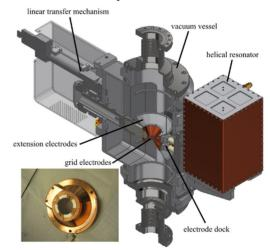
Figure 2: Retractable grid-based buncher hardware.
