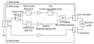
Figure 5: Bunching system block diagram.
