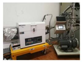
Figure 2: Quantitative deposition coating system.
