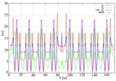
Figure 1: Twiss functions for the double mini-betay lattice in the TPS storage ring.
