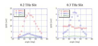
Figure 7: THz intensity and beam angle relationship. MC2: Photon Sources and Electron Accelerators A23 Other Linac-Based Photon Sources corresponds to the Cherenkov angle. Furthermore, the assumed frequency was enhanced at each slit, and we have successfully confirmed the quasi-monochromatization.
