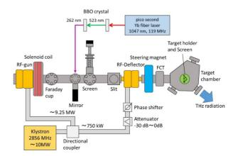
Figure 5: Experimental setup of monochromatic coherent terahertz radiation using electron beam tilting.
