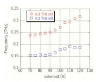
Figure 6: Corresponding frequency to solenoid current relationship.
