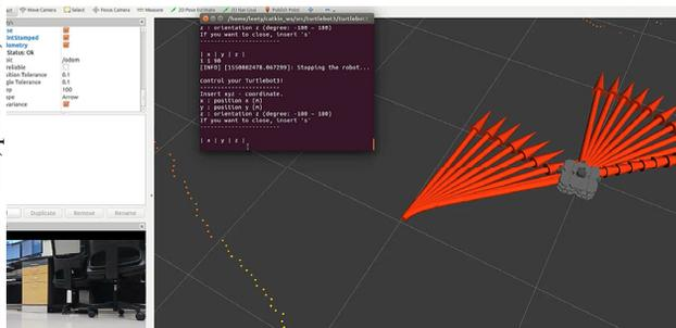
Figure 3: Point operation: the robot can be moved by 2D point (x, y) and z-angular. The red arrows show which direction it's facing while it's moving.
