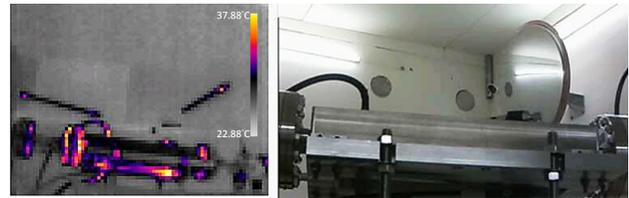
Figure 10: Thermal image of a strip line kicker.
