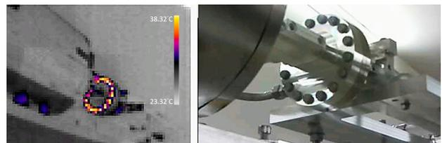
Figure 12: Thermal image of a flange.
