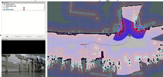
Figure 5: The navigation enables a robot to move from the current pose to the designated goal pose on the map. The
