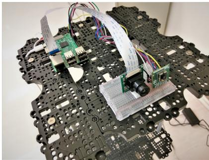
Figure 8: A Pi camera and a thermal imaging module (FLiR Dev Kit) were hooked up with another Raspberry Pi.
