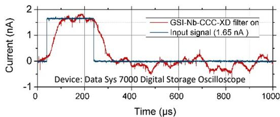
Figure 4: Pulse signal response of (#3) with SQUID electronics and 10 kHz low-pass filter switched on [9].
