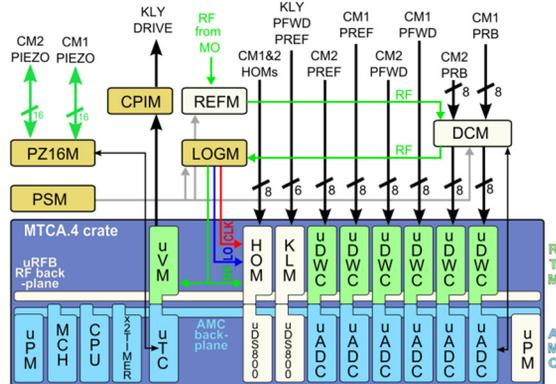
Figure 2: Schematic of a LLRF system of the Eu-XFEL.
