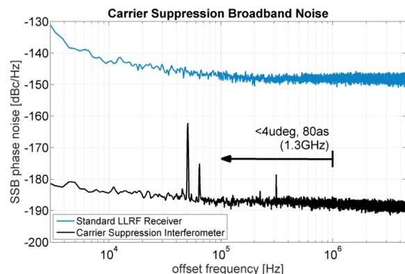
Figure 7: Carrier suppression resolution of about 80 as within 1 MHz, @ 1.3 GHz, +17 dBm power level (black), currently used non-IQ field receiver (blue).
