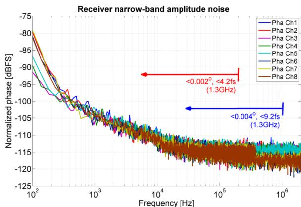
Figure 1: Field detector narrow-band phase noise with 0.002 deg, 4.2 fs (100 Hz - 200 kHz), respectively 0.004 deg, 9.2 fs(100Hz - 1 MHz) @ 1.3 GHz.
