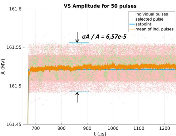
Figure 4: Amplitude in-loop performance at FLASH.
