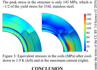
Figure 3: Equivalent stresses in the coils (MPa) after cooldown to 1.9 K (left) and at the maximum current (right).
