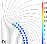
Figure 2: HTS insert fields (T) in 15 T dipole (A), in outer coils only (B) and stand-alone with/without iron yoke (C-D).
