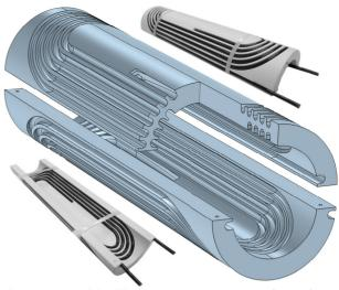
Figure 1: Double-COMB support structure (center) and the mock-up coil (top and bottom).
