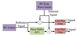
Figure 6: Simplified block diagram of an I/Q demodulator.
