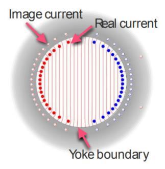
Figure 2: Cosine  $\theta$  magnet concept.
