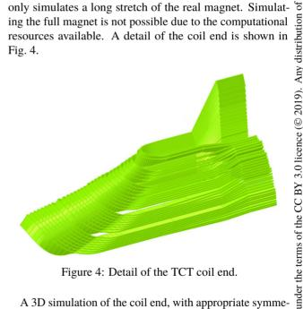
Figure 4: Detail of the TCT coil end.
