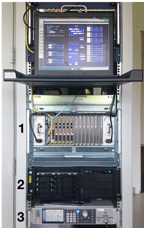
Figure 3: LLRF System for LILAC, Assembled for Sytem Integration at MicroTCA Technology Lab, consisting of: 1) MicroTCA-Crate, 2) External CPU, 3) Master Oscillator.
