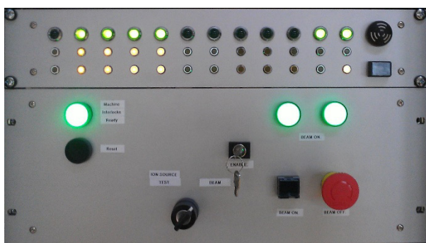
Figure 6: Machine interlock and control status panel.
