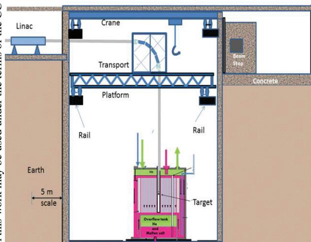
Figure 2: Underground placement of Linac and Reactor.
