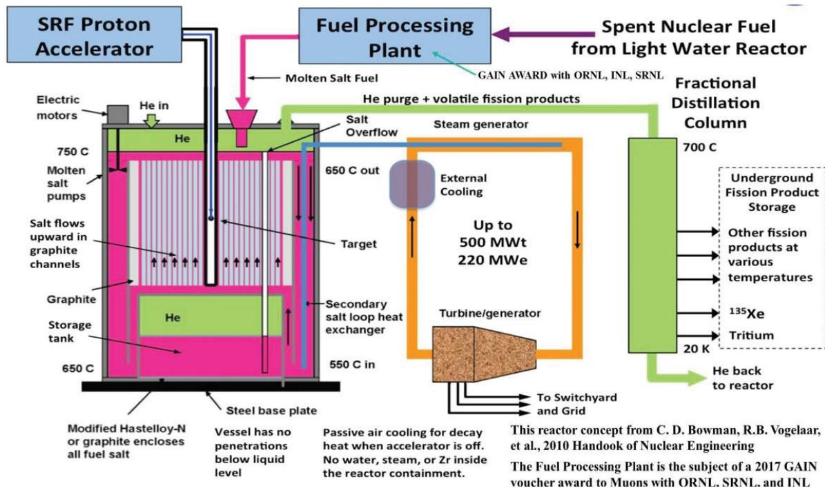
Figure 1: Conceptual diagram of the Mu\*STAR system, comprised of a 1 GeV, 2.5 MW SRF proton Linac, a 500 MWt graphite moderated reactor with internal solid metal spallation neutron target, a molten-salt fuel preparation plant, and collection system for volatile radioisotopes. The reactor power can be used for process heat or electricity generation.
