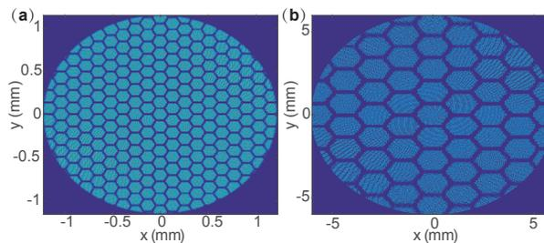
Figure 2: Simulated first stage (a) and second stage (b) images of a virtual 200 mesh TEM grid.
