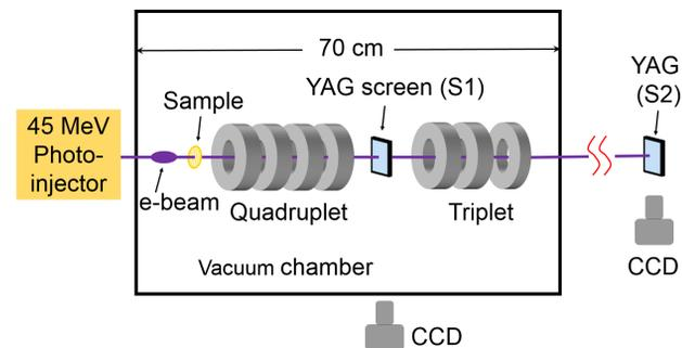
Figure 3: Schematic of the CHEER experiment.
