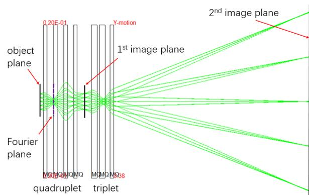
Figure 1: Electron trajectory tracking in CHEER using COSY INFINITY [15].
