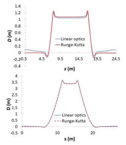
Figure 4: Dispersion function of the RAFFIA at injection energy (upper) and extraction energy (lower).
