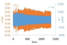
Figure 5: The beam size during acceleration in horizontal direction monitored at the QF and vertical direction monitored at QD.
