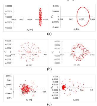
Figure 7: The Poincare map of the beam core evolution observed at the injection point for (a)  $I_B = 50 \ \mu\text{A}$ , (b)  $I_B = 200 \ \mu\text{A}$ , and (c)  $I_B = 250 \ \mu\text{A}$ .
