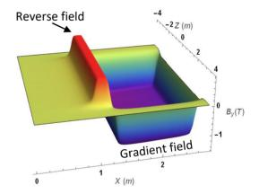
Figure 1: Designed magnetic field data on the median plane.
