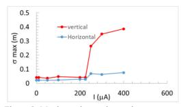
Figure 8: Maximum beam size vs. beam current.
