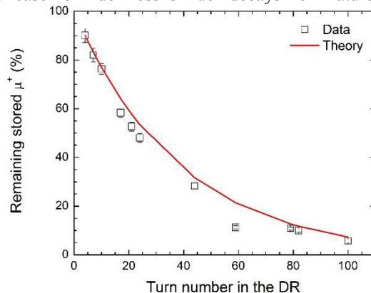
Figure 3: Percentage of stored muons in the g-2 ring versus the DR turns. Red curve is the exponential decay law.
