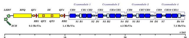
Figure 6: Layout of the HELIAC accelerator.
