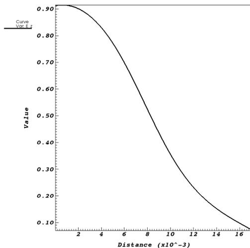
Figure 3: Electric field along the axis of the TW cavity.
