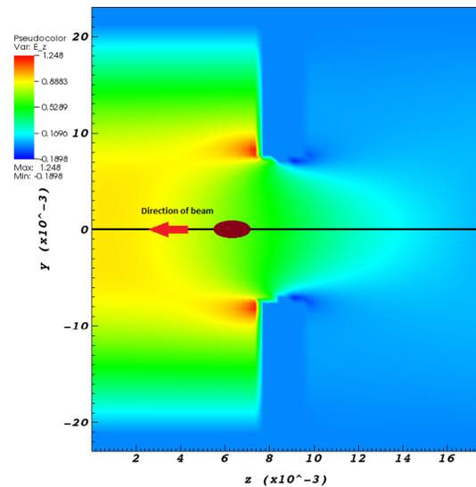
Figure 2: Electric field distribution in the C-band structure corresponding to the fundamental mode at 5.712 GHz.
