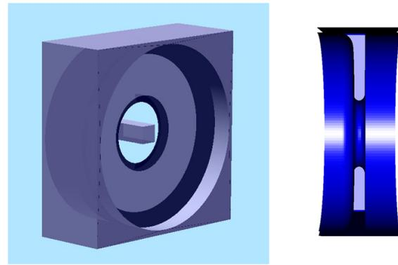
Figure 1: Model of a traveling wave, C-band structure and the cross section view.
