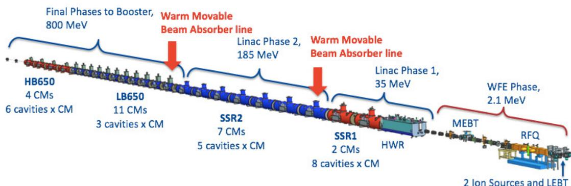
Figure 1: 3D Model of the ~215 m long PIP-II accelerator from the two  $H^-$  ions sources (right) to the HB650 section (left). Beam Commissioning Phases are shown as well as the proposed Warm Movable Beam Absorber locations: at the first SSR2 CM (to allow the Linac Phase 1 Beam Commissioning) and at the first LB650 CM (to allow the Linac Phase 2 Beam Commissioning).
