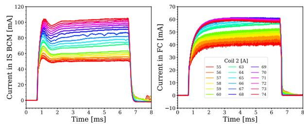
Figure 2: Beam pulse changes during a Coil 2 scan. Magnetron power, Coil 1 current, Coil 3 current, and H<sub>2</sub> injection were kept to 500 W, 120 A, 217 A, and 3.5 sccm.
