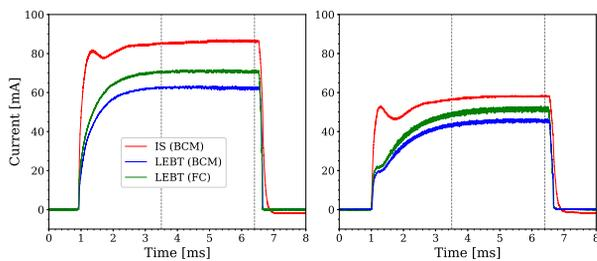
Figure 4: Beam pulses for the Standard Setting and Low Setting. The dotted lines indicate the 2.9 ms plateau.
