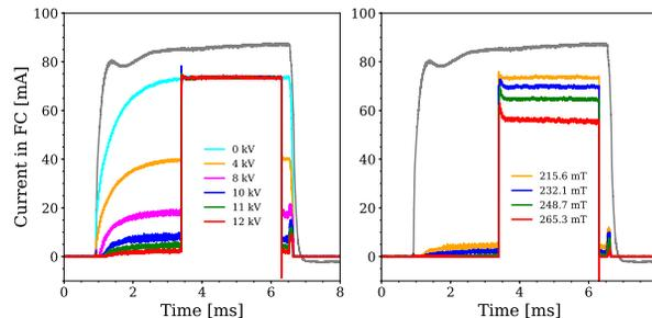
Figure 6: Chopped beam pulses for different chopper voltages (left) and different solenoid 2 strengths (right). The grey trace is the IS pulse as a reference.
