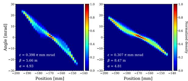
Figure 5: Preliminary EMU measurements in Permanent Tank for the Standard Setting and Low Setting.
