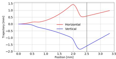
Figure 2: Beam trajectory under the influence of the Earth magnetic field. The black vertical dashed line marks the interface LEBT-RFQ.
