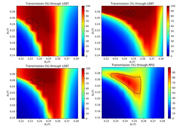
Figure 6: Transmission through the LEBT. Dashed lines show 25% and 50% mismatch for (top left) initial emittance of  $0.25 \pi$  mm mrad, (top right) SCC level reduced to 90% and (bottom left) initial emittance of  $0.25 \pi$  mm mrad and SCC reduced to 90%. (bottom right) Transmission through RFQ using a beam with emittance of  $0.25 \pi$  mm mrad and SCC level of 90% in the LEBT. Dashed line shows the contour of the transverse emittance at  $0.25 \pi$  mm mrad.
