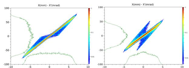
Figure 1: Old (left) and new (right) IS distributions from the IBSimu code.
