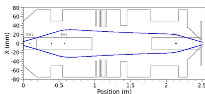
Figure 3: Update LEBT aperture geometry, together with  $2 \times \text{RMS}$  beam envelope.
