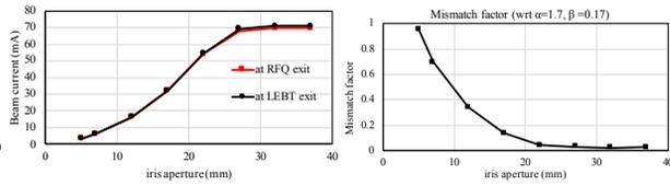
Figure 5: Output current and mismatch factor at the LEBT exit with respect to the iris aperture radius.
