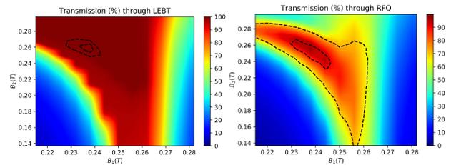
Figure 4: Transmission through the LEBT (left), with dashed lines showing 25% and 50% mismatch. Transmitted particles through the LEBT and RFQ (right), with dashed lines showing the contour of the transverse emittance at 0.15 and  $0.25 \pi \text{ mm mrad}$ .
