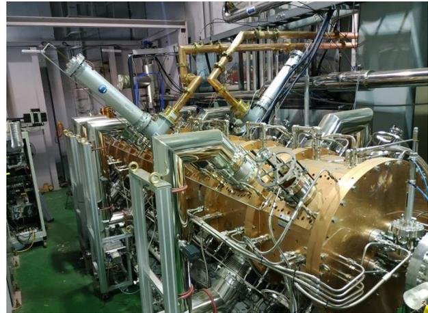
Figure 4: Two power couplers were installed and each will be connected to 80 kW SSPA systems.
