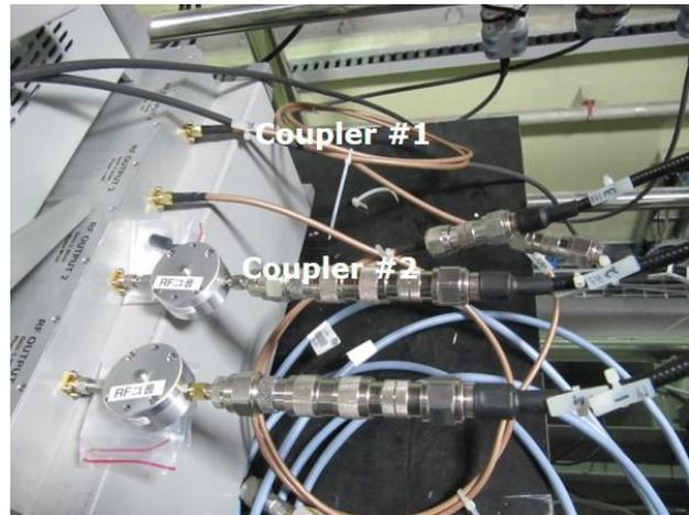
Figure 5: Phase difference between two power couplers was compensated by the cable length of the low power level and phase shifters.
