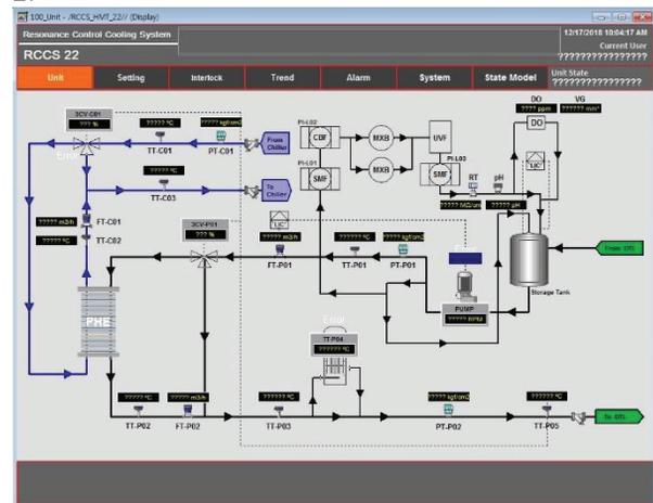
Figure 2: Piping and instrument diagram.
