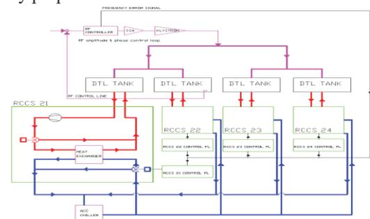
Figure 3: 20MeV radio frequency control scheme.
