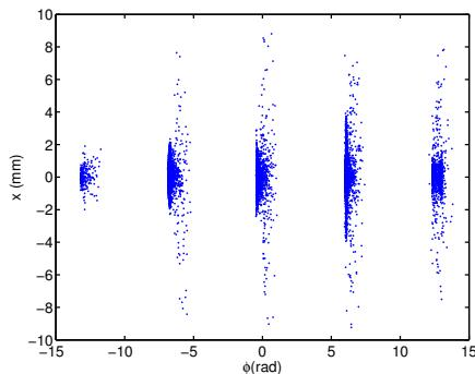
Figure 5: Micro-bunches at the exit of the bunching system.
