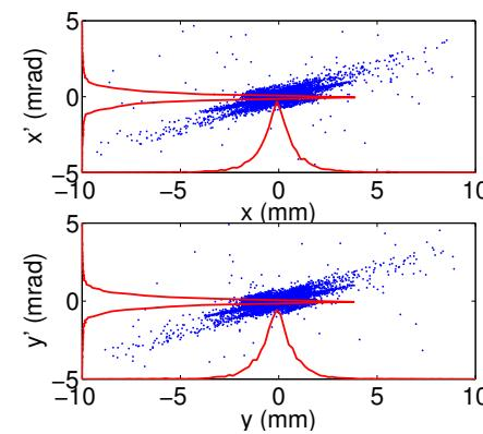
Figure 4: The electron distribution at the exit of the bunching system. (left)x-x'phase space; (right)y-y'phase space.
