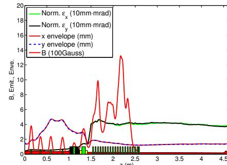
Figure 3: The distribution of magnetic field, normalized emittance and envelope of the selected solution along the beam line.
