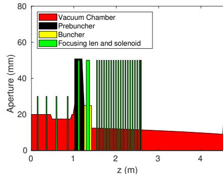
Figure 1: Layout of the bunching system of the HEPS linac.
