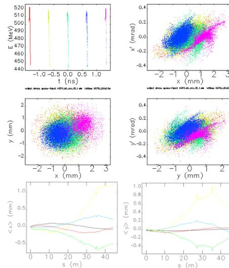
Figure 4: The beam distribution at the Linac exit (top) and beam orbit (bottom) of Scheme I.
