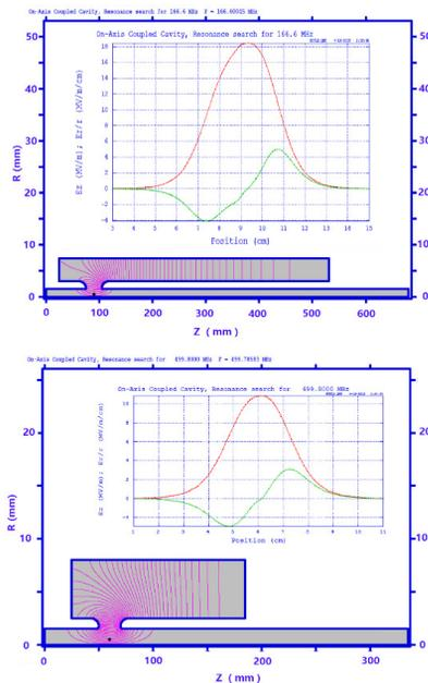
Figure 2: The schematic and electric field distribution of SHB1 (top) and SHB2 (bottom).
