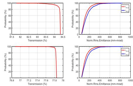
Figure 6: The transmission and emittance with misalignment errors and orbit correction. The top figures show the results of total beam and the bottom figures show the results of the beam within  $\pm 1.5\%$  energy spread.
