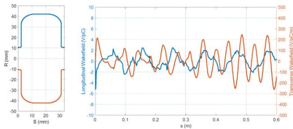
Figure 3: The cell shape and long-range Wakefield of one cell in accelerating structure.
