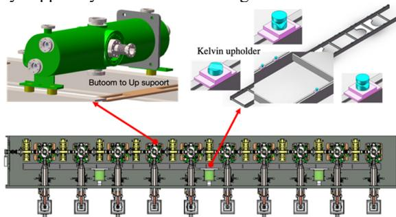
Figure 7: Specific mechanical structures for superconducting cavity support system.
