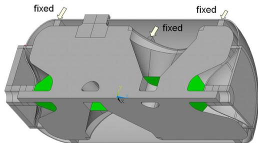
Figure 3: Spoke042 cavity structure. Green parts are extra stiffening at nose and spoke.
