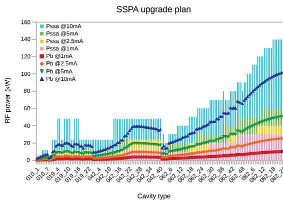
Figure 4: SSPA upgrade plan.
