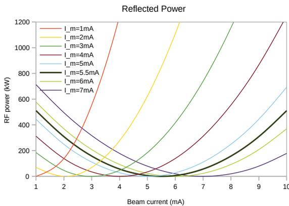
Figure 2: Reflected RF power ratio at different  $P_{b,m}$ .
