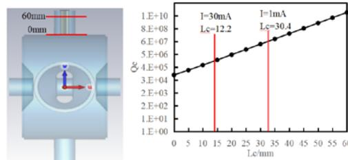
Figure 6: Inserting antenna length vs.  $Q_e$ .
