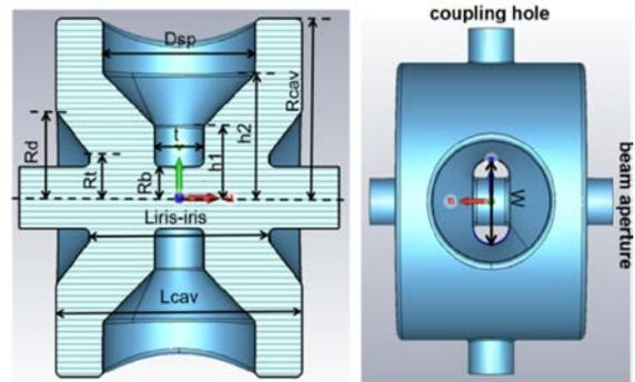
Figure 2: Geometrical parameters of 648MHz single spoke cavity.
