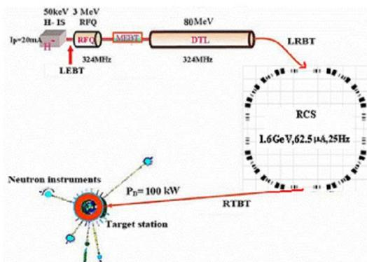
Figure 1: Schematic layout of the CSNS.
