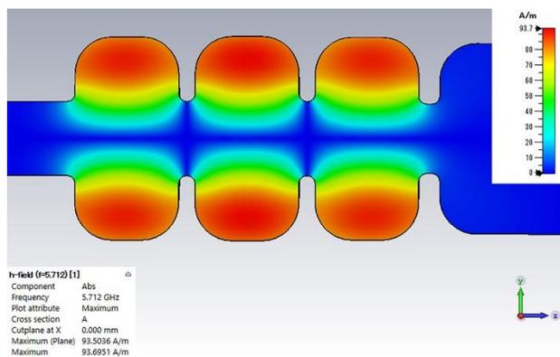
Figure 2: Magnetic field distribution in the accelerating cells which resulted from the CST Studio simulation.
