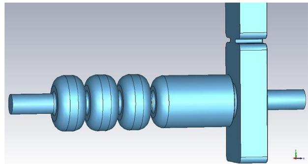
Figure 1: A 3D drawing of the 3-cell cavity designed for high-power and high-gradient experiments.
