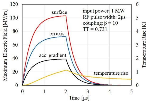
Figure 4: The build-up of the electric field and the temperature rise of the cavity surface resulting from the pulsed heating simulation at an input peak RF power of 1 MW for 2  $\mu$ s.
