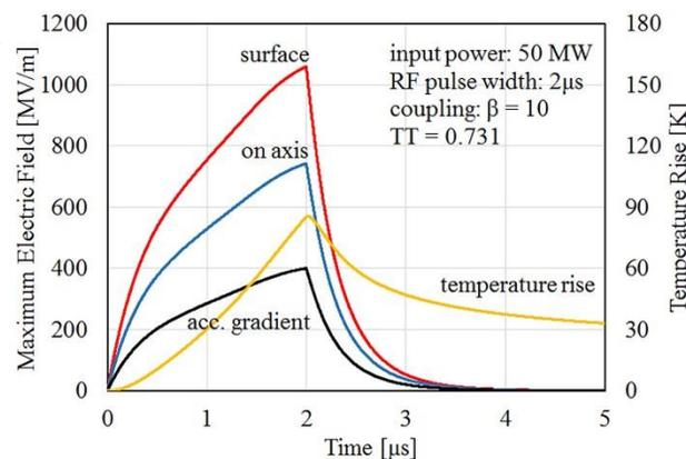
Figure 5: The build-up of the electric field and the temperature rise of the cavity surface resulting from the pulsed heating simulation at an input peak RF power of 50 MW for 2  $\mu$ s.
