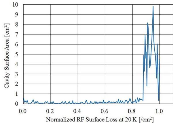
Figure 3: Distribution of the cavity surface area as a function of the normalized RF loss per unit area over the entire surface of the accelerating cells.
