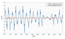
Figure 7: Vertical dispersion before and after coupling correction.
