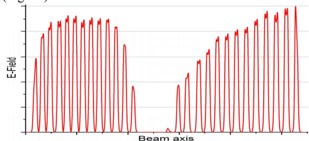
Figure 8: Simulated electrical field distribution along the beam line.
