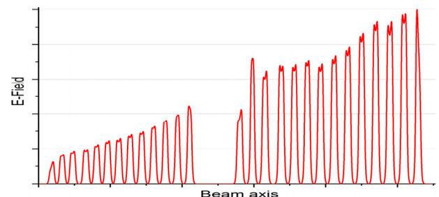
Figure 9: Simulated electrical field distribution along the beam line with tuning bodies.
