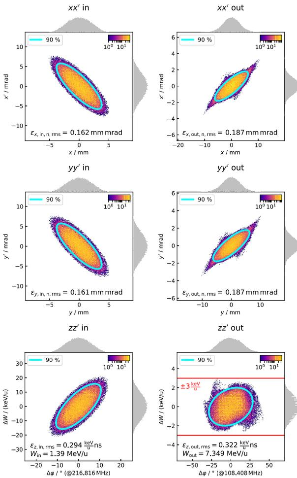
Figure 5: Simulated transverse and longitudinal phase space portraits downstream the HELIAC for the nominal case. The particle density is logarithmically color-coded.
