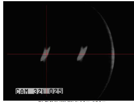
Figure 8: Screen picture from a 50/50 kicked an unaffected beam at micro pulse level at 100 kHz beam rate.
