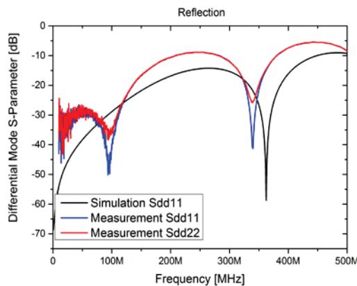
Figure 4: Comparison of measured S11 and S22 parameters in diff. mode excitation with the CST simulation.
