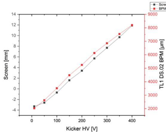
Figure 7: Displacement of the electron beam after 7 m at the magnetic septum as a function of HV.
