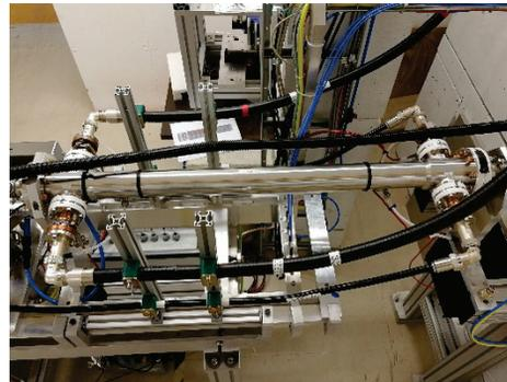
Figure 6: Picture of the kicker installation on the ELBE beam line.
