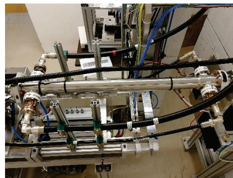
Figure 6: Picture of the kicker installation on the ELBE beam line.
