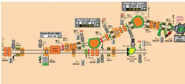
Figure 9: Schema of the beam lines (ELBE operator interface). Neutron (upper beam line) and Laser interaction (straight beam line) are branching at the septum.
