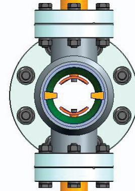
Figure 2: Sectional drawing of the ELBE kicker in the area of the connection ports.
