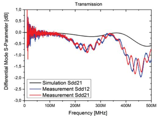
Figure 5: Comparison of measured S12 and S21 parameters in diff. mode excitation with the CST simulation.
