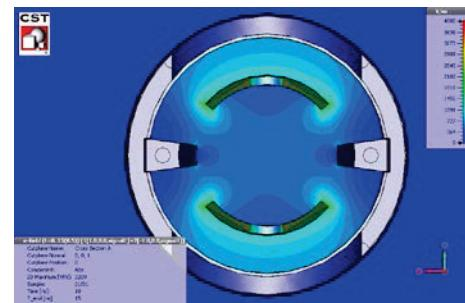
Figure 3: Sectional plot of the electric field in the medium section of the kicker structure.
