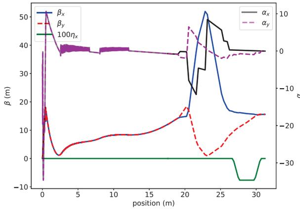
Figure 4: The Twiss parameter evolution is illustrated along the length of the linac. The bunch compressor terminates at  $z \sim 31$  m, the plasma is anticipated to be located at  $\sim 34$  m.
