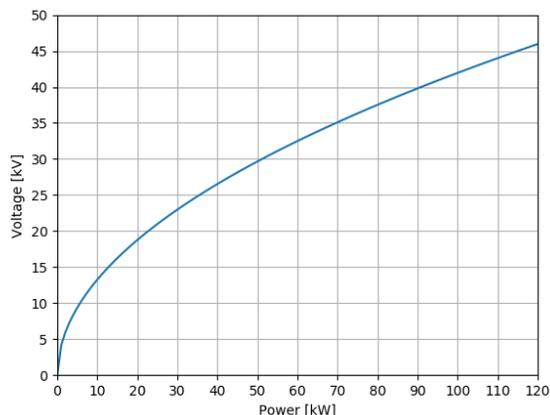
Figure 4: The calculated electrode voltage of the RFQ against the power.
