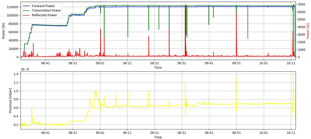
Figure 3: Measured power and pressure data for the commissioning of the MYRHHA-RFQ up to 120 kW.
