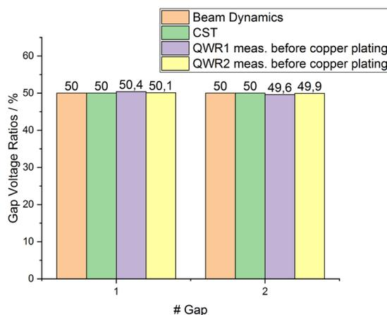
Figure 2: Comparison of the gap voltage ratios for QWR 1 and QWR 2.
