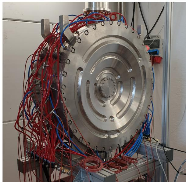
Figure 4: CH 1 in the bunker of the experimental hall of the IAP with connected vacuum and cooling water system including temperature monitoring.
