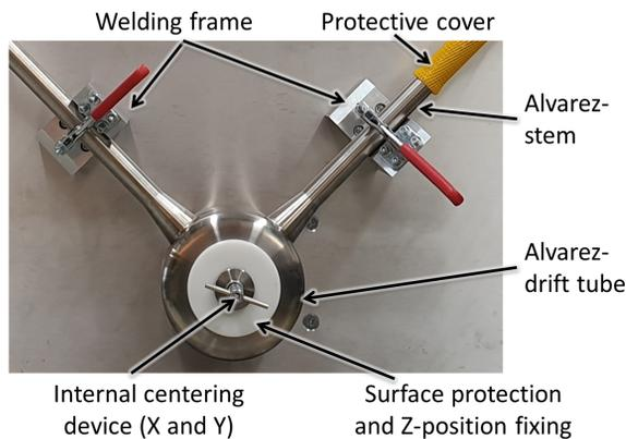
Figure 5: Empty drift tube for RF tests produced at GSI mechanical workshop. The picture shows the drift tube in the last welding frame for welding on the stems.
