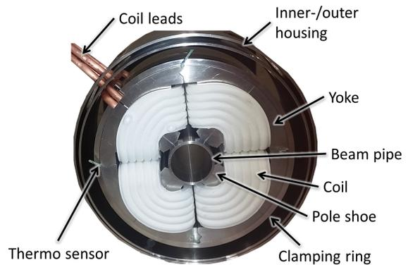
Figure 4: Mechanical development of the first prototype drift tube including a dummy magnet with 3D printed coils.
