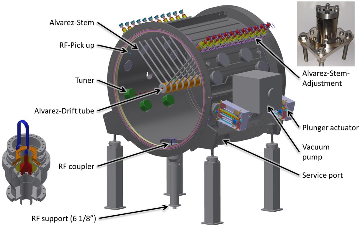
Figure 3: CAD-model of the Alvarez-FoS cavity section with a length of 1.9 m and 11 drift tubes. The drift tubes are installed at the top of the tank, but other combinations are possible. The bottom houses RF coupling, a support hole. Vacuum pumps and pickups are installed (light blue) at the side.
