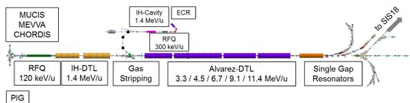
Figure 1: Schematic overview of the GSI UNILAC.
