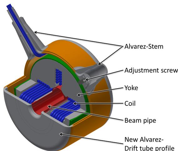
Figure 6: CAD-model of the integrated quadrupole singlet.
