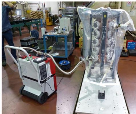
Figure 2: Leak test of section.
