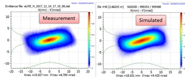
Figure 7: Phase space distribution in the MEBT, comparison for the 5 mA  $\text{H}^+$  beam.
