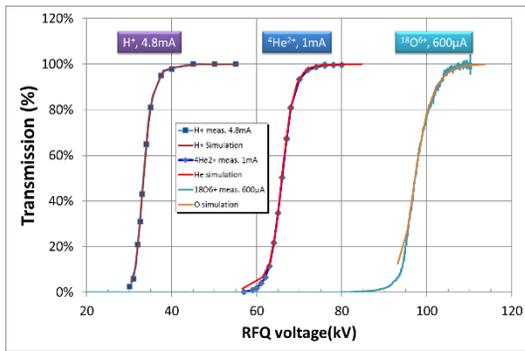
Figure 3: Transmission of the 3 reference particles.
