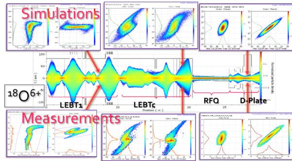
Figure 6: Comparison between simulations and measurements for the transverse emittance of the  $^{18}\text{O}^{6+}$  beam in the LEBT and MEBT lines ( $650\mu\text{A}$ ).
