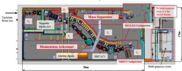
Figure 4: S3 experimental hall with the two-stage optical structure including the main elements - dipoles, Superconducting Multipole Triplet (SMT), detection systems - and the different focal planes ( $F_i$  with  $i = 0-4$ ): target point  $F_0$ , momentum dispersive plane  $F_1$ , achromatic focal plane  $F_2$ , energy dispersive plane  $F_3$ , final focal plane  $F_4$ .
