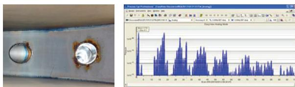
Figure 2: Internal oxidation of a vacuum chamber on welded seams and residual vacuum spectrum of an elastomer component not compatible with ultra-vacuum.
