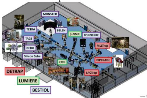
Figure 5: Overview of the DESIR experimental platform. A central beam line delivers the radioactive ions to experimental devices grouped into three subsets: DETRAP (in red), LUMIERE (in green) and BESTIOL (in purple).
