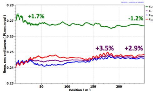
Figure 3: RMS emittances through the SC linac.
